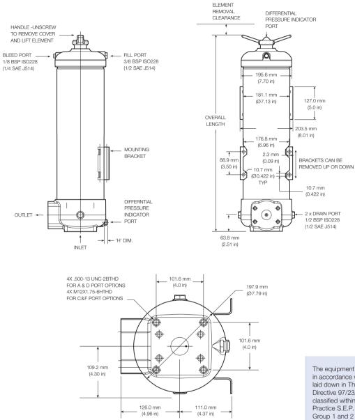
The equipment has been assessed in accordance with the guidelines laid down in The European Pressure Directive 97/23/EC and has been classified within Sound Engineering Practice S.E.P. Suitable for use with Group 1 and 2 fluids only. Consult Sales for other fluid gas group suitability.
